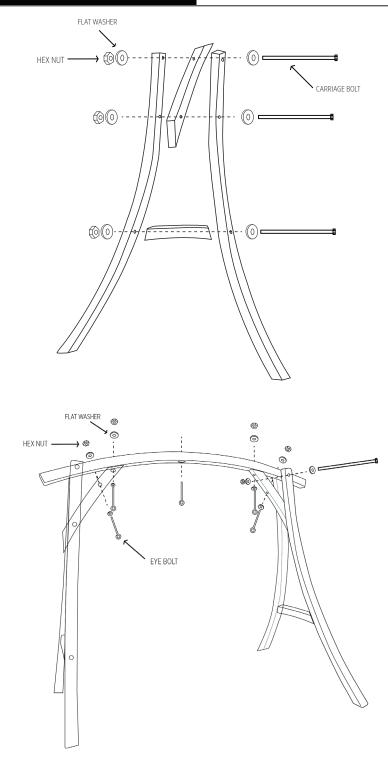
**STEP 1.** Insert (3) Hex bolts, (6) flat washers (one on each side), and (3) hex nuts into the top, middle, center section of beams. Repeat on each side. The top center beam should hand lose until step 2.
